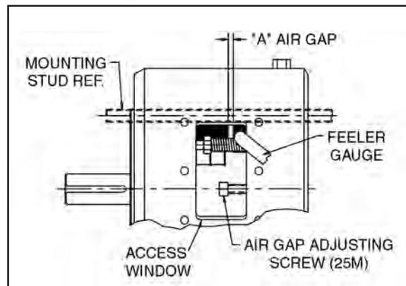
3. Turn two square head adjusting screws (25M) until air gap "A" measures:
